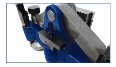
Improvements to the equaliser pivot section prevents the pin from rotating and this eliminates casting wear. Pin head recessed into the casting to minimise free play along its axis.
